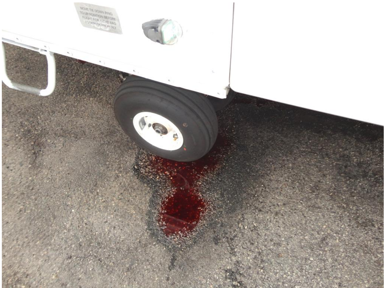
Figure 15: Leaked Hydraulic Fluid
