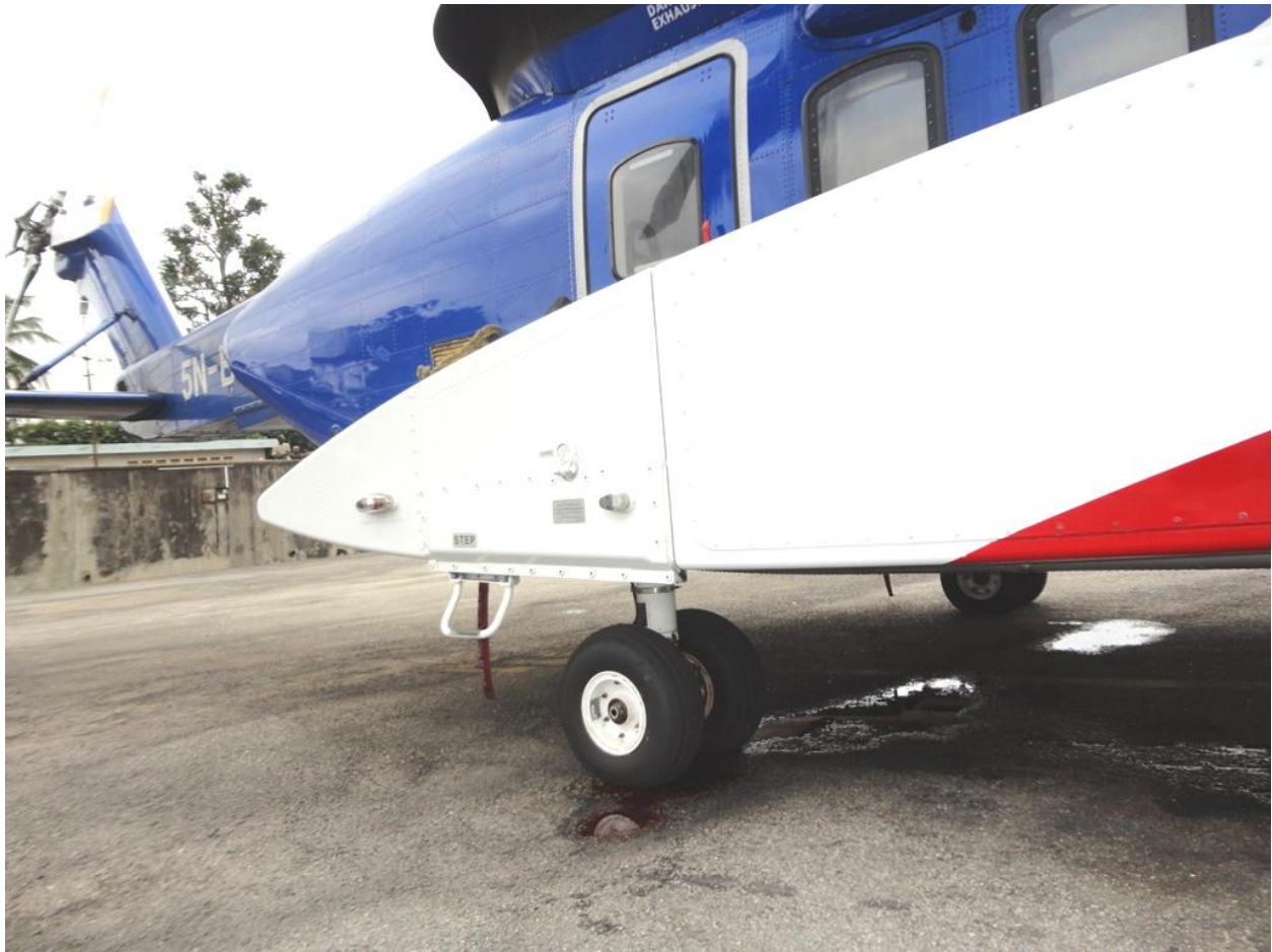
Figure 16: Leaked Hydraulic Fluid
