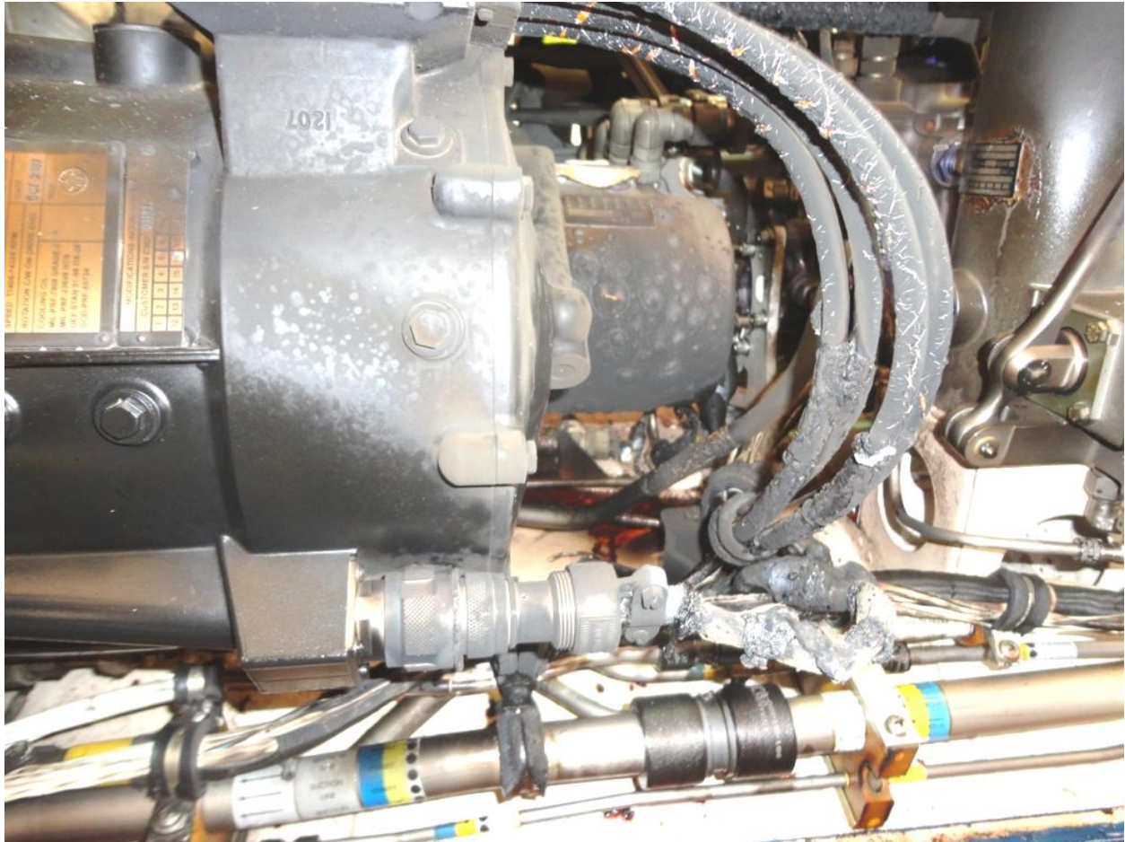
Figure 17: Burnt Out Area around the Heat Exchanger
