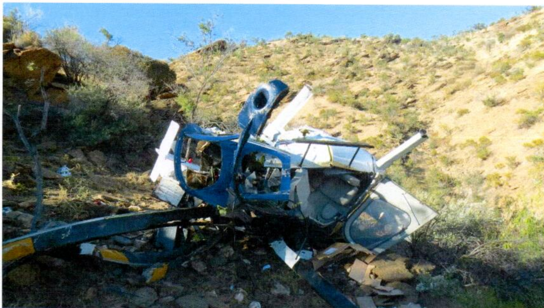
Figure 3. Depicting aircraft inverted position with cabin livable space reduced.
